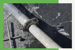
Be aware of the "Hazard Zones" around a pump. These include the charge hopper, the reduction elbow, hoses, clamps and pipes. Due to equipment malfunction or metal fatigue, they are all common points of failures.
